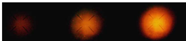
Fig. 4. True color fluorescence image of a Rhodamine-labeled DNA array on Au exposed to buffer (left), salmon sperm, which approximates a random DNA assortment (middle) and the complimentary sequence (right). The substrates were excited at 514 nm and the images were obtained on an inverted optical microscope. The intensity ratio of the fluorescent spots is 1:3:30.
